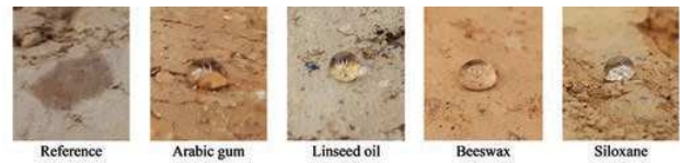
FIGURE 4 Examples of water droplets on top of treated and untreated rammed earth specimens during the microdrop absorption time test.
