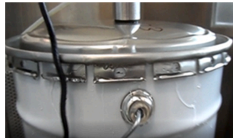
Fig. 5. Deformations in hydraulic pressure tests.
