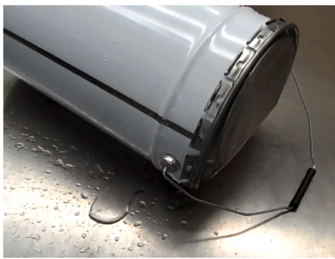
Fig. 31. Packaging with new edge after drop test on the top.
