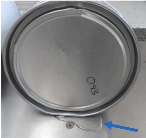
Fig. 3. Packaging after the oblique drop test on the bottom.
