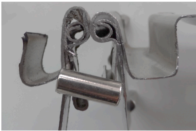
Fig. 30. Section of the closure deformed by the drop test on the bottom (left) compared with a closure from an untested package (right).
