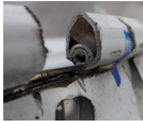
Fig. 9. Cut in the deformed closure area by drop test on the bottom.
